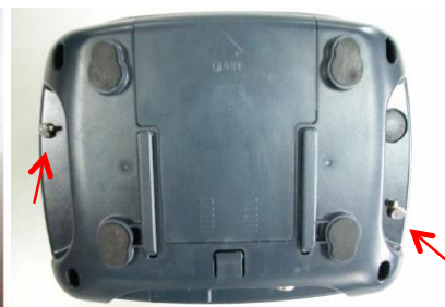
Sealing with lead seals
